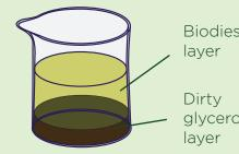
The used oil is reacted with alcohol to create biodiesel and glycerol, which separate into layers.
